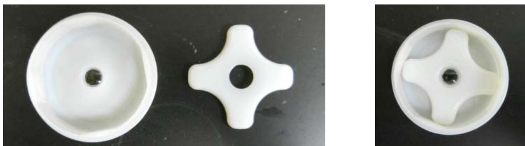
Figure 3.2: Custom Corneal Holder. Left: Picture of the Anchoring Top and the Base Disassembled. Right: Picture of Anchoring Top and Base Assembled.
