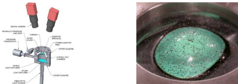
Figure 2.4: Left , Schematic of a corneal inflation rig. Right , Picture of a Bovine Cornea placed onto an Inflation Rig (Boyce et al. 2008).
